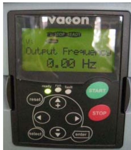
NXS (model of frequency inverter) keypad.
