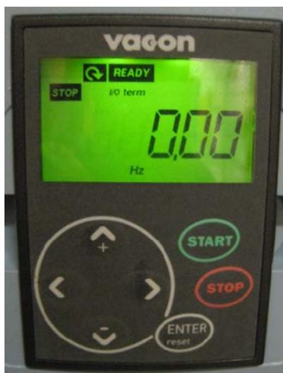
NXI (model of frequency inverter) keypad.
